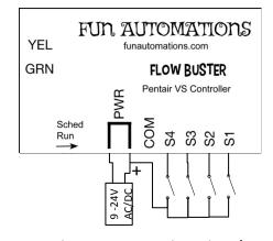
Or by connecting the relays/ switches to the power supply. Positive side if using DC, Either side if AC. If The Negitive side of the DC is connected the unit won't be damaged, it just will not operate when the contacts are closed.
