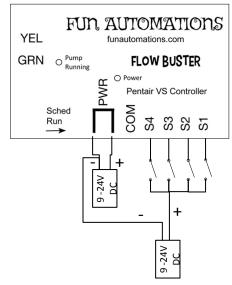
Or also by using a second power supply, ONLY IF USING DC, by connecting the negatives together and the positive to the switches/relays.
